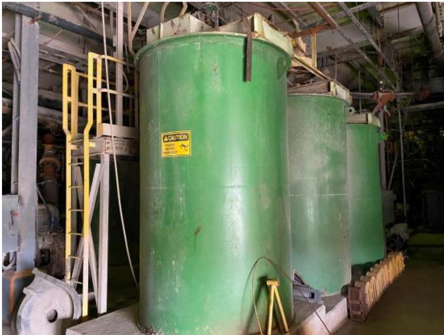
Figure 18-42: Reagent Tanks
