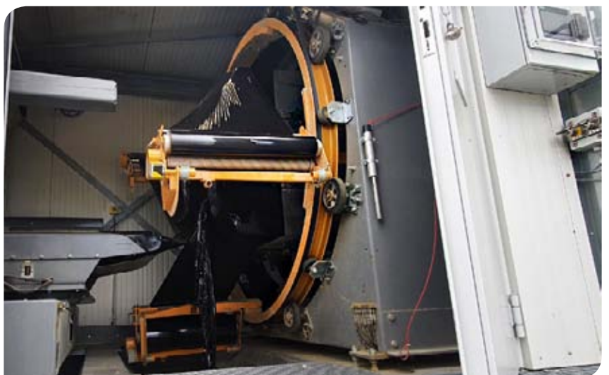
Below: View of the wrapping step.
